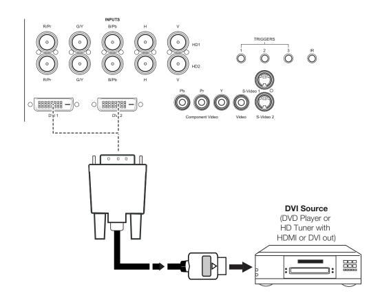
Figure 3-5. DVI Source Connections
